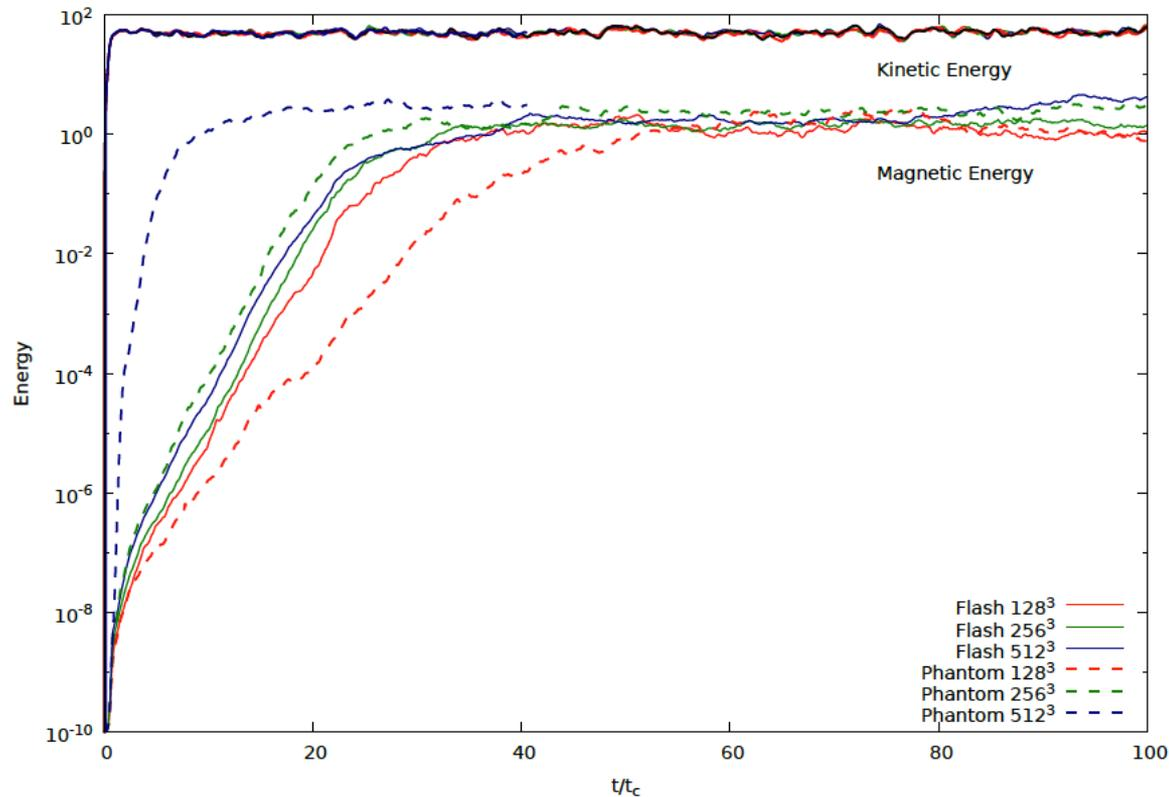
**Figure 1.** Growth and saturation of the magnetic energy for FLASH and PHANTOM at resolutions of  $128^3$ ,  $256^3$ , and  $512^3$ . The top lines are the kinetic energy for the six calculations. FLASH has similar growth rates across the resolutions simulated, while PHANTOM exhibits faster growth rates with increasing resolution. This resolution dependence is a consequence of the artificial dissipation terms. Both codes saturate the magnetic energy at similar levels.
