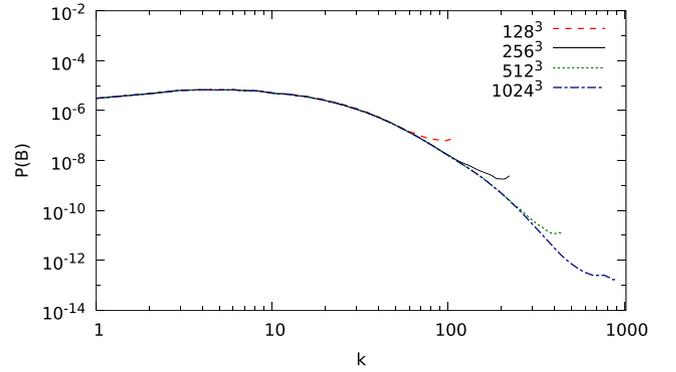
**Figure A2.** Conversion of a  $128^3$  particle PHANTOM snapshot to grids of resolutions from  $128^3$  to  $1024^3$  grid points. Each resolution agrees well on the large-scale structure, but captures more of the small-scale structure as the resolution is increased. We find that the  $256^3$  resolution grid sufficiently captures the total magnetic energy, therefore, we choose grids with double the number of grid points as particles for our analysis.
