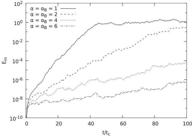
**Figure 4.** A  $128^3$  PHANTOM calculation where the artificial viscosity and resistivity parameters are systematically increased (no switches are used). With increasing dissipation, the growth rate decreases, producing the same behaviour consistent with changes in resolution.
