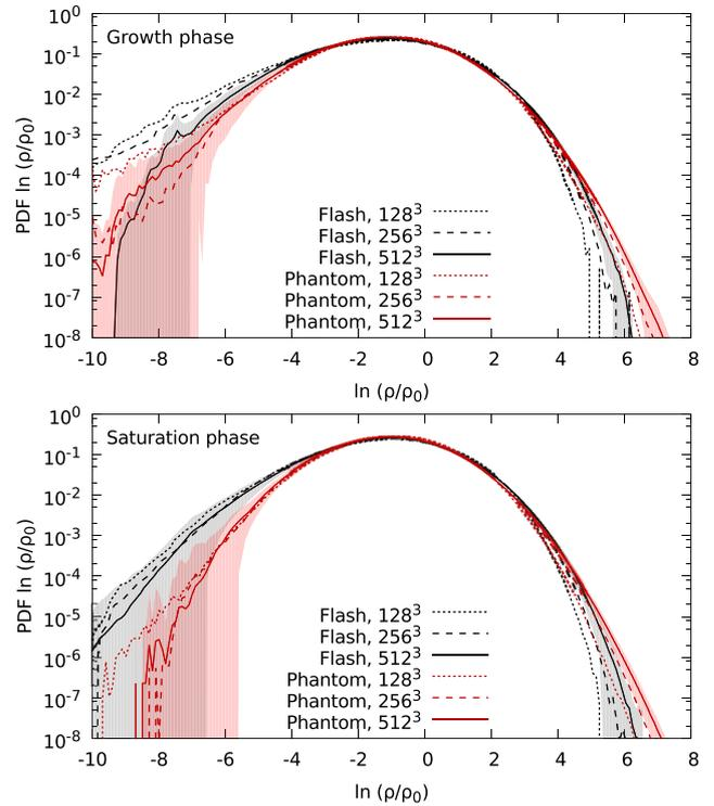
**Figure 12.** Time averaged density PDFs during the growth phase (top panel, for  $t/t_c = 2-10$ ) and during the saturation phase (bottom panel, for  $t/t_c = 30-100$ , only  $t \geq 50$  for the  $128^3$  PHANTOM calculation). The peaks and high-end tail of the PDF are similar for both cases, but the low-density tail is less extended when the magnetic field has reached saturation.
