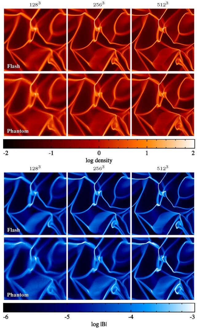
**Figure 1.** Slices of  $\rho$  (top) and  $|B|$  (bottom) in the  $z = 0.5$  mid-plane at  $t/t_c = 1$  during the initial formation of the turbulence. The results from FLASH (top row) and PHANTOM (bottom row) are shown for resolutions of  $128^3$ ,  $256^3$ , and  $512^3$  (left to right). As the resolution is increased, the shock lines become more well defined. The regions with highest magnetic field strength are in the dense shocks.
