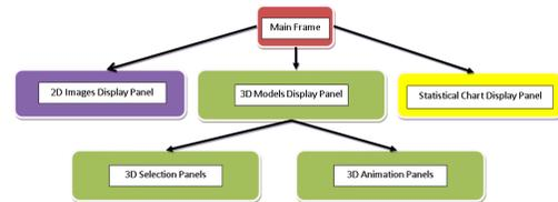
Visualization architecture. The main frame consists of a 2D display panel, a 3D display panel, and a statistical chart panel. More details of 3D models can be seen by selecting a 3D sub-volume or initiating animation.
