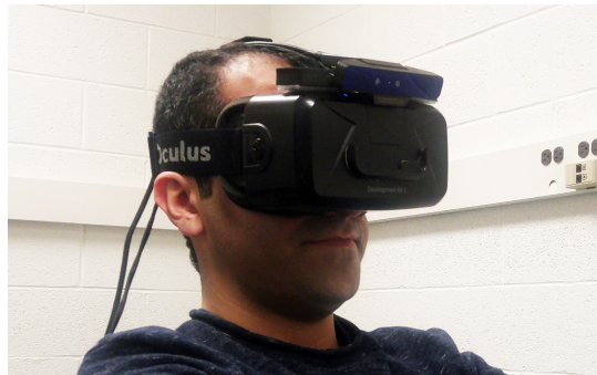
Fig. 1. User wearing a RealSense RGBD camera on an Oculus HMD.
