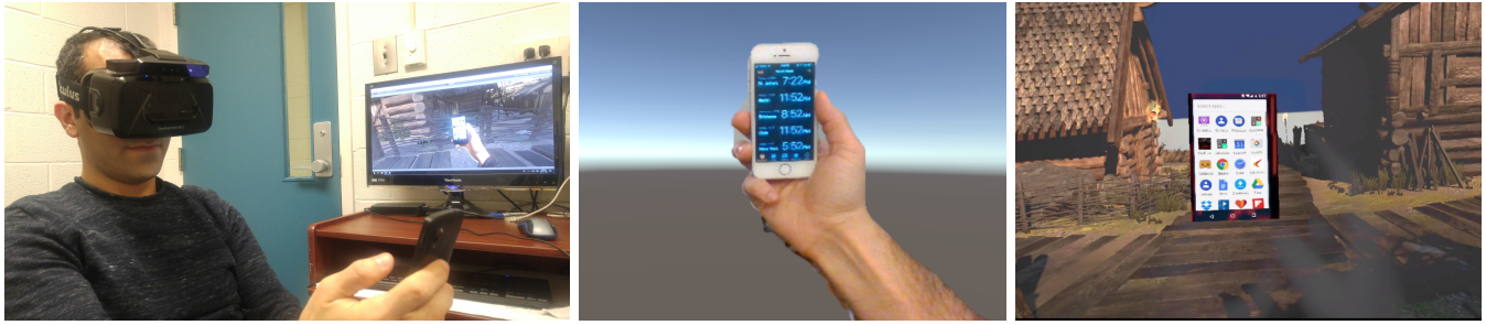
Fig. 2. Near-Range Augmented Reality: On the left, a user holding a phone in front of the HMD. In the middle, an image of the users's hand and phone as it appears within the default virtual environment. On the right, Augmented Reality as it appears when using SDSC.
