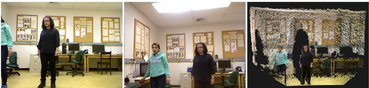
**Figure 5:** An example of successful registration of a multi user scene where one camera is located higher than the other one.
