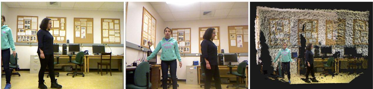
**Figure 4:** Example result of two users where half of one user is captured by one camera and the full body is captured by the other.
