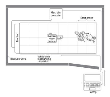
Fig. 1. Overhead schematic diagram of the test apparatus. Not to scale.
