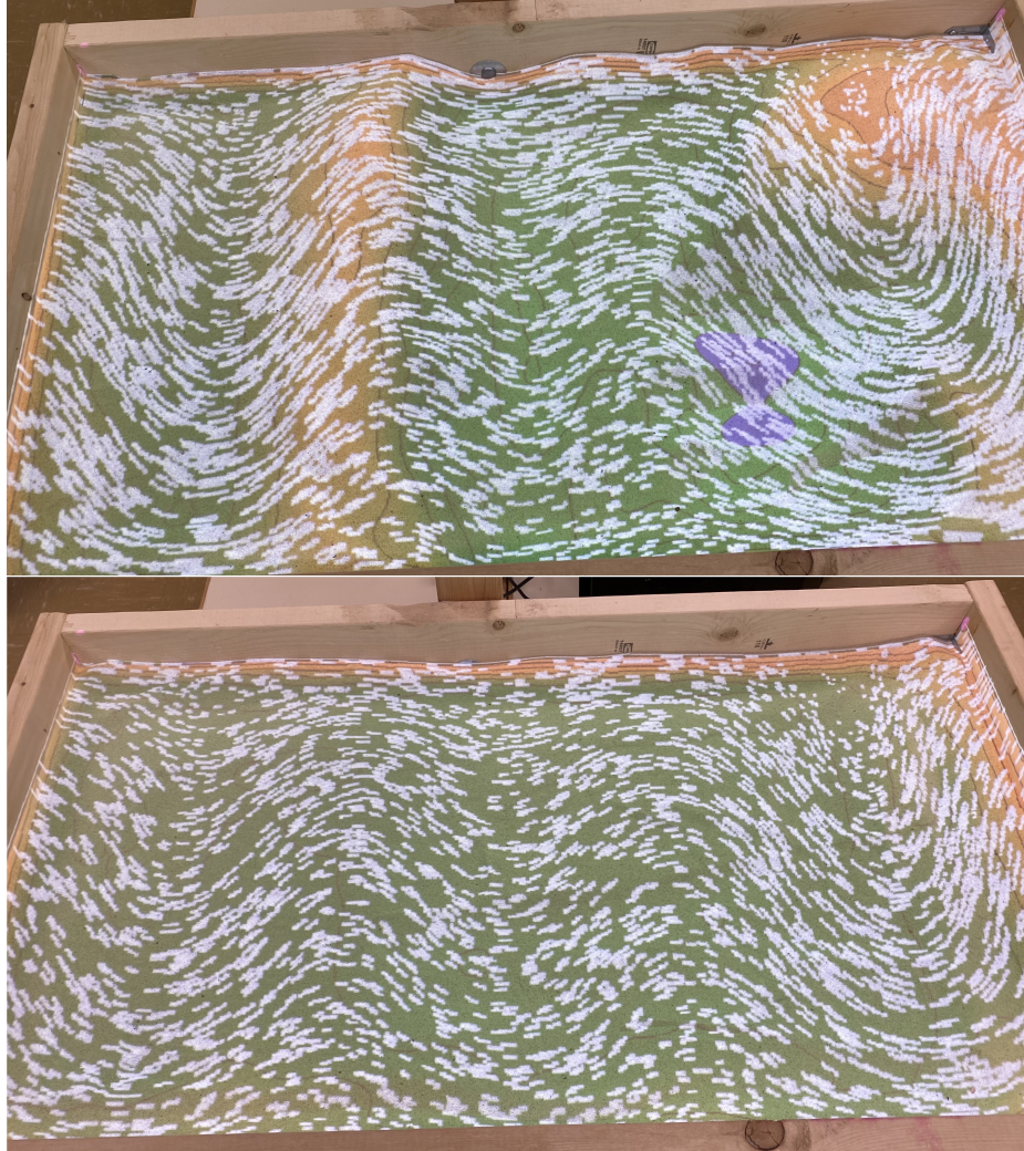
Figure 4.9: The final visualization using the Charney & Eliassen model. The top image has bumpy terrain; the bottom image has flat terrain
