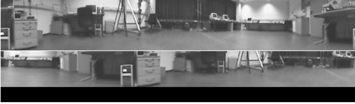
Figure 9: Images from the A1OriginalH database taken at location (1,1). Top image shows the original image taken by the robot. Bottom image shows the image after a random amount of rotation, plus a random vertical shift. The remaining pixels after vertical shifting are filled in with black.
