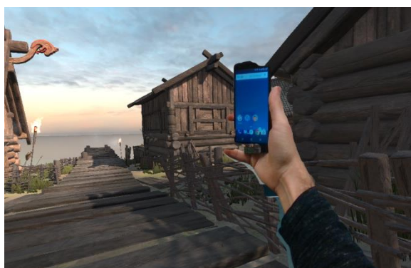
State 3: Incorrect segmentation with flickering effect and not detecting the borders of the smartphones or part of the user's hand correctly.
