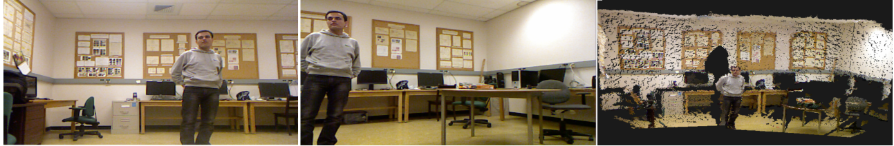
Figure 1: Successful registration of two viewpoints sharing small amount of overlap (The two figures on the left show RGB images, and the right figure shows the registered point cloud).
