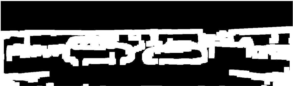
Figure 2.10: Dilation of the detected edges in Figure 2.7 with a 10x10 structuring element
