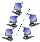
shared wire (e.g., cabled Ethernet)
