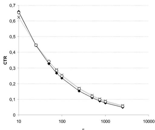
Fig. 6. Critical transmitting range in the stationary case and with intermediate RWP mobility ( $p = 100$  and  $p = 200$ ) for values of  $n$  ranging from 10 to 2,500. The  $x$ -axis is in logarithmic scale.
