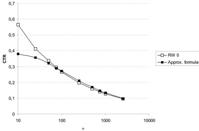
Fig. 7. Critical transmitting range with RWP mobility when  $p = 0$  (RW 0) and values of the CTR as computed with our formula (Approx. formula). The values of  $n$  range from 10 to 2,500, and are reported in logarithmic scale.
