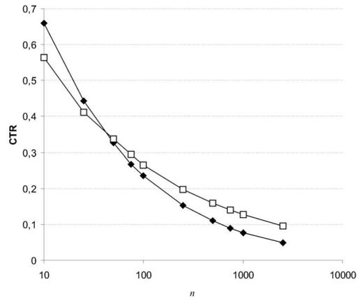
Fig. 5. Critical transmitting range in the stationary case and with extreme RWP mobility for values of  $n$  ranging from 10 to 2,500. The  $x$ -axis is in logarithmic scale.
