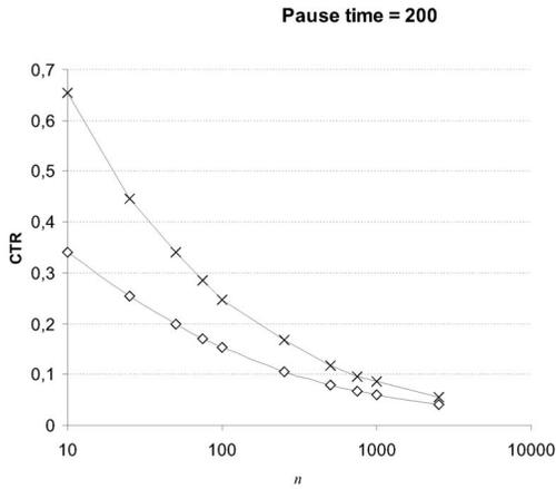
Fig. 4. Theoretical and experimental value of the critical transmitting range for values of  $n$  ranging from 10 to 2,500 when the pause time is set to 200 and  $v_{min} = v_{max} = 0.01$ . The  $x$ -axis is in logarithmic scale.
