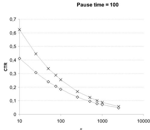
Fig. 3. Theoretical and experimental value of the critical transmitting range for values of  $n$  ranging from 10 to 2,500 when the pause time is set to 100 and  $v_{min} = v_{max} = 0.01$ . The  $x$ -axis is in logarithmic scale.
