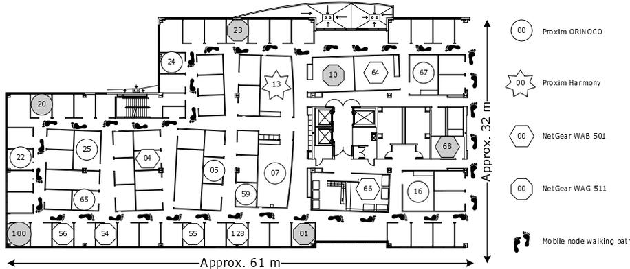
Figure 2: Our testbed consists of 23 nodes placed in fixed locations inside an office building. Four different models of 802.11a wireless cards were used. The six shaded nodes were used as endpoints for a subset of the experiments (see section 5.3). The mobile node walking path shows the route taken during the mobility experiments (see section 6).
