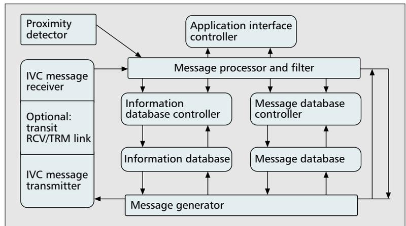
■ Figure 3. The communication subsystem of a message relay box.
