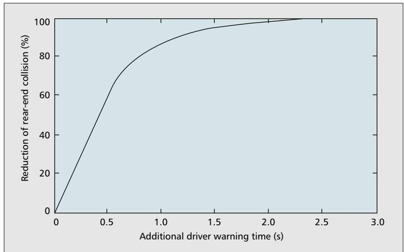
■ **Figure 1.** Providing a driver with an additional 1 s of warning time to react can reduce rear-end collisions by nearly 90 percent [2].
