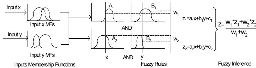
Figure 7: TSK fuzzy inference system structure.
