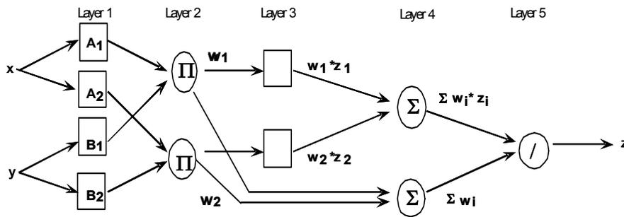
Figure 8: The ANFIS system architecture.
