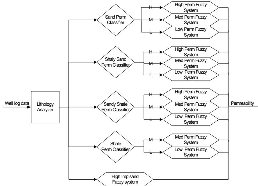
Figure 4: The hybrid system high-level structure.
