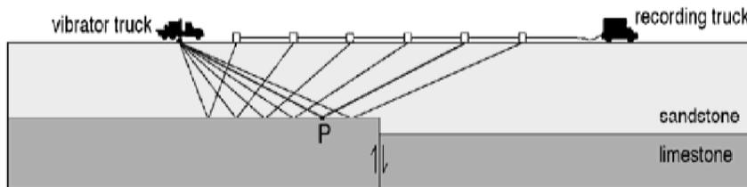
Figure 1. Schematic of the seismic method.
