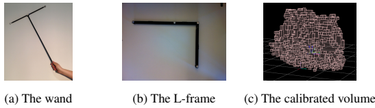
Figure 1: The calibration wand (a) features two reflexive markers placed on a T-shaped rod, while four static reference points are arranged on an L-shaped frame (b). As the distance between the markers is predefined, the system can be calibrated by analysing the view of the wand and the L-frame from multiple cameras. This results in a finite volume (c) where the system can reliably provide positional information.
