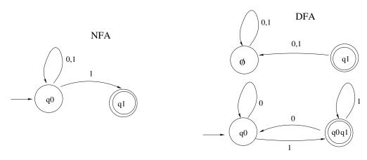
To formalize this intuition, let's describe  $D(Q', \Sigma, \delta', q_0, F)$ . We will have to talk about sets of states reachable from a given set by following  $\epsilon$ -arrows: let's call, for a set of states  $Q_i$ , a  $E(Q_i) = \{q \in Q | \exists q' \in Q \text{ such that } q \text{ is reachable from } q' \text{ by following } \epsilon\text{-arrows}\}.$
