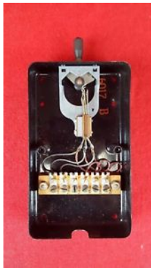
Electromechanical Telephone Switch (1930s)
