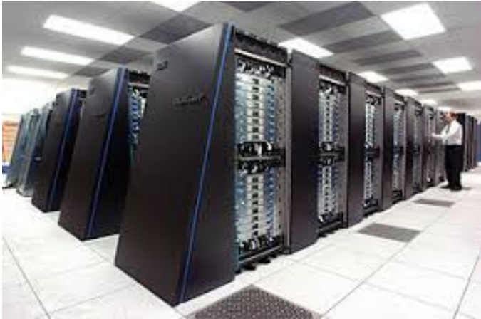
IBM Blue Gene/P (2007) [164K processor cores]
