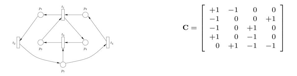
• A Petri net is defined by sets of places (representing conditions) and transitions (representing events) which are connected to each other by directed arcs,  $\mathcal{N} = (P, T, A)$ . We define:
