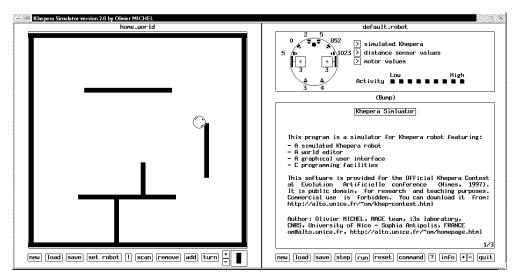
Figure 9. The Khepera simulator. A small robot navigating in a random environment.
