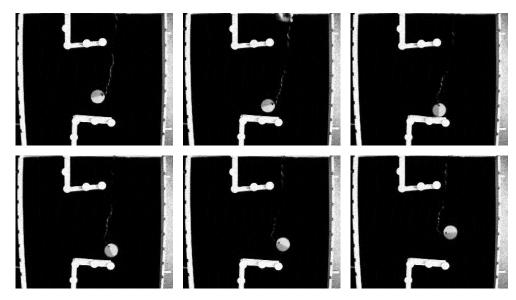
Figure 12. Movement of a real Khepera robot. The Khepera encounters a wall and turns counterclockwise (top left to bottom right). Wide-angle view of a top-mounted camera looking down on a  $1-m^2$  test maze.
