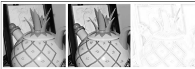
Fig. 6.25 Unsharp blur filter: evolved filter, GIMP filter and difference image.
