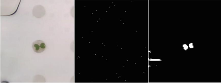
**Fig. 3.7** The results of using pixel-based random selection on one of the KOMATSUNA images. The image is shown on the left. In the middle, the 40 sampled pixels are shown, as selected using random selection. On the right, the segmentation pattern is shown
