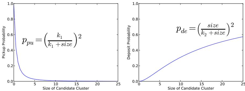
**Fig. 3** The pick-up (left) and deposit (right) probabilities as functions of cluster size. The dashed lines indicate the particular choices of parameters utilized in our experiments ( $k_1 = 1$ ,  $k_2 = 8$ ).
