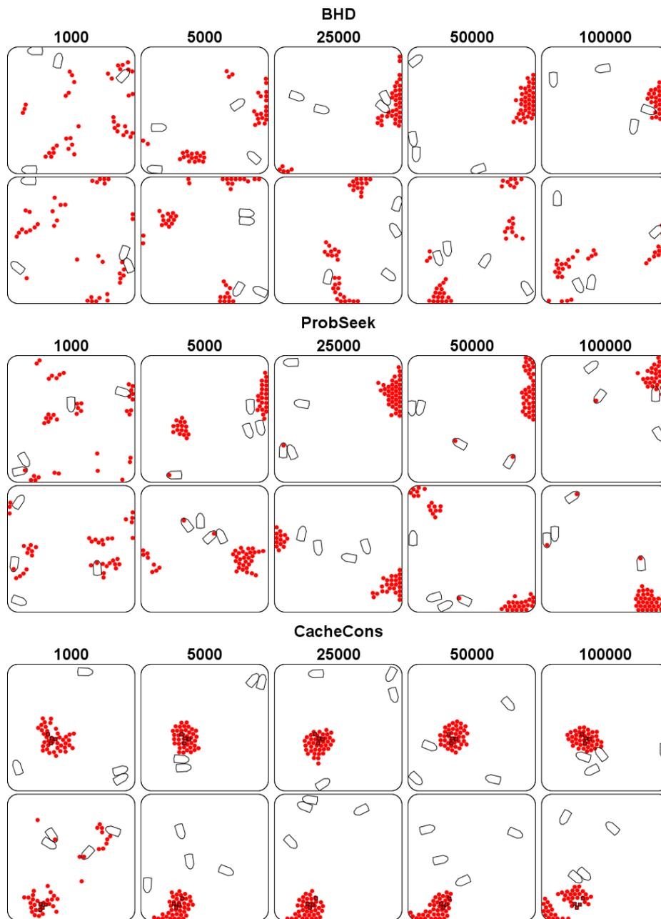
**Fig. 8** Snapshots of the performance of BHD, PROBSEEK, and CACHECONS operating on 40 pucks of one type. Snapshots from the first two of 20 trials are shown in each row. Cache points for each robot are shown as filled squares. The position of the robots at the time of each snapshot is also indicated. Note that in some cases the robots are carrying pucks. (Colour figure available online)
