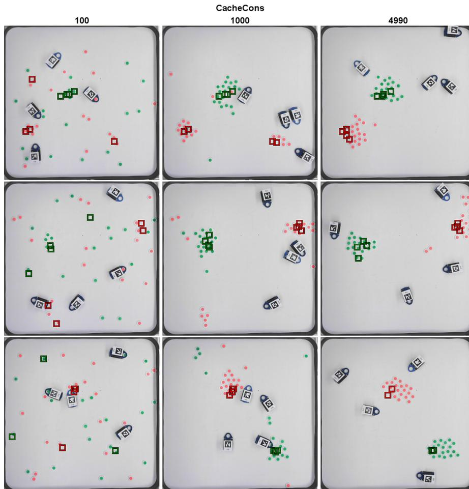
**Fig. 15** Snapshots from all three live trials of CACHECONS. Coloured squares indicate the cache points of each robot. (Colour figure available online)
