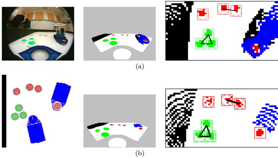
**Fig. 2** This figure shows the view from one of our SRV-1 robots (a) and a simulated robot (b). In (a) the robot’s raw view, colour segmented image, and local map are shown from left-to-right. In (b) an overhead view of the simulator is shown, the simulated robot’s raw view (no colour segmentation is required), and the local map. (Colour figure available online)
