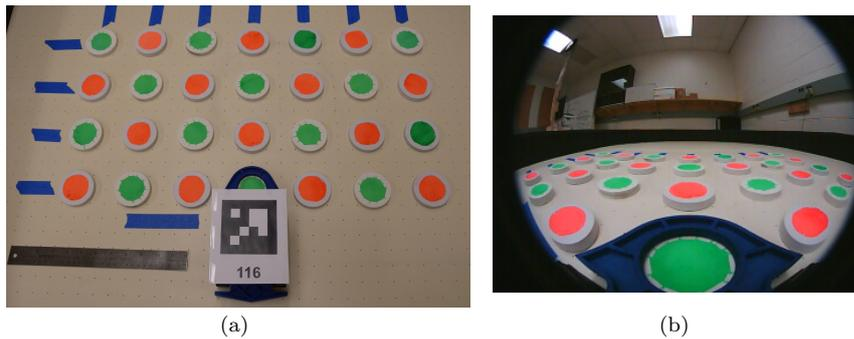
**Fig. 6** Views of the calibration grid from overhead **(a)** and from the robot **(b)**. (Colour figure available online)
