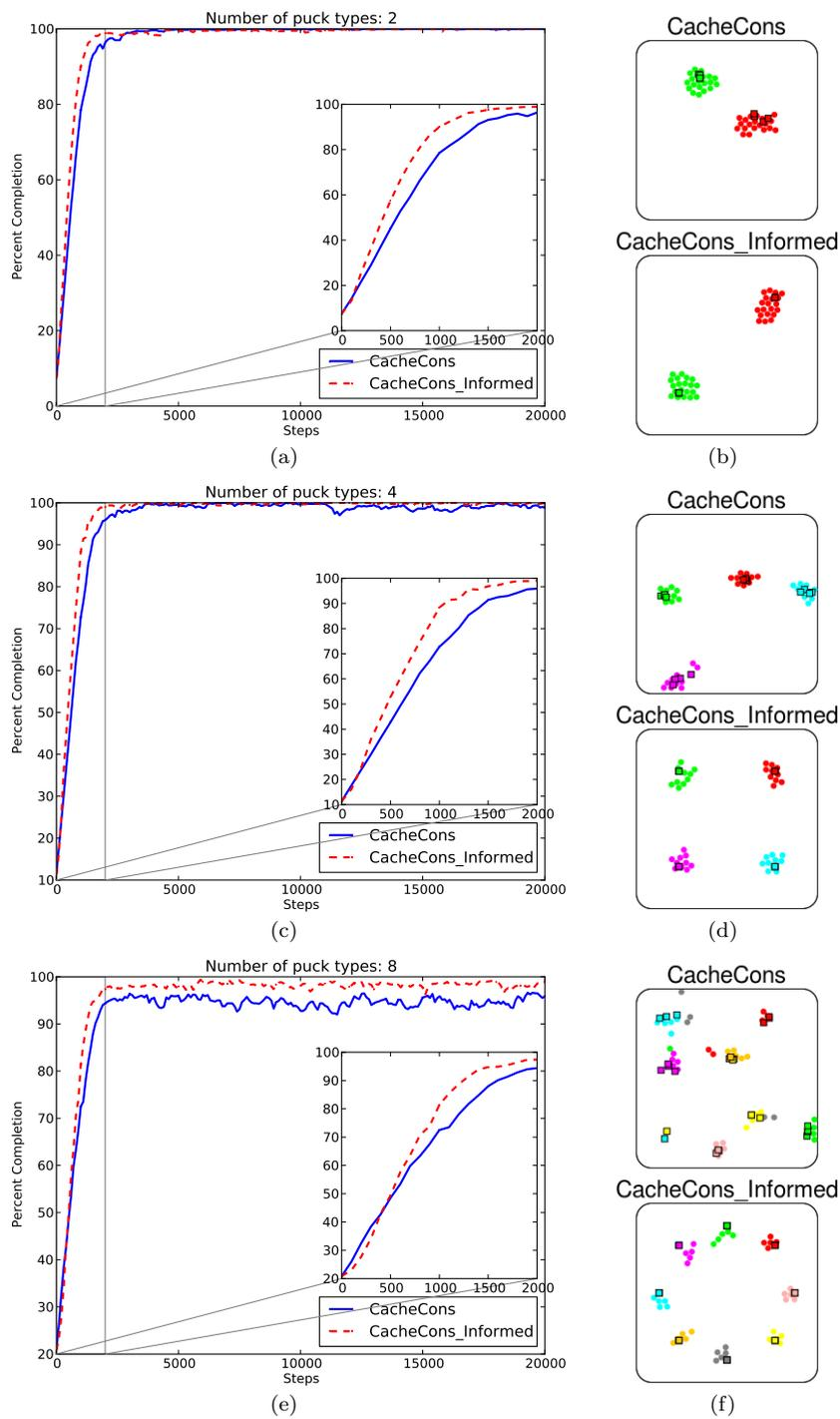
**Fig. 12** (a), (c), and (e): Percentage completion plots for CACHECONS versus CACHECONS.INFORMED for 2, 4, and 8 object types. (b), (d), and (f): Snapshots captured at 2,000 time steps. (Colour figure available online)
