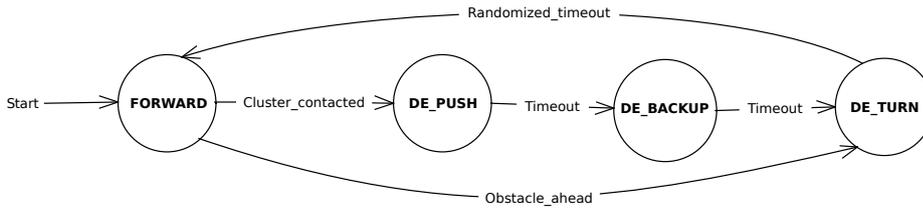
**Fig. 4** Finite state machine for BHD.
