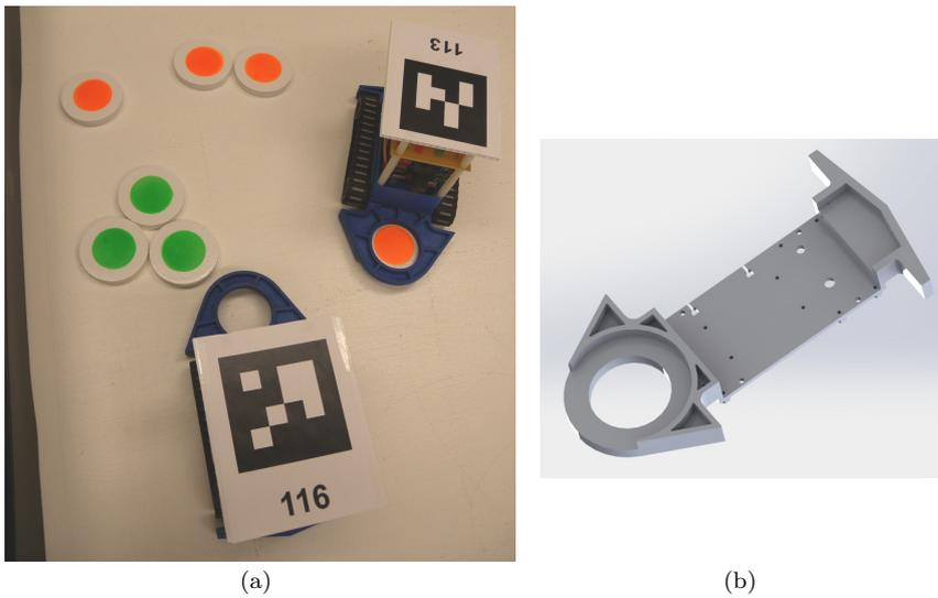
**Fig. 1** (a) Two of our modified SRV-1 robots in operation. Views from robot ‘116’ are presented in Figure 2(a). (b) The underside of the robot’s housing, showing the shape of the passive gripper. (Colour figure available online)
