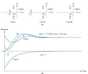
If the third pole is near the other two then its effect is strong. However, as it is moved to the left it decays at a faster rate and therefore has less effect on the overall signal. Even if the exponential decays quickly, we may still be concerned about its initial effect. Actually, the effect of the third pole decreases in magnitude (as well as decay rate) as the pole moves to the left. Consider again the system response:
