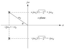
$\sigma_d = \zeta \omega_n$  is the real part of the pole and is called the *exponential* decay frequency.
