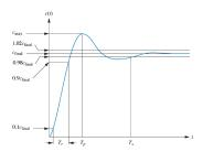
Consider determining  $T_p$ , the time required to reach the first peak. At the peak, the derivative is zero. Thus, we can solve for the value of t for which  $\dot{c}(t) = 0$ . We do this differentiation in the FD:
