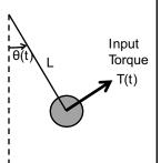
$$\left[\begin{array}{c} x_1(t) \\ x_2(t) \end{array}\right] = \left[\begin{array}{c} \theta(t) \\ \dot{\theta}(t) \end{array}\right] \quad mL^2 \ddot{\theta}(t) + mgL \sin(\theta(t)) = T(t)$$
