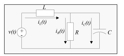
Step 1 Select the <u>state variables</u>: write the derivative equation for the energy-storage elements (L and C)...
