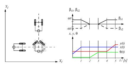
During time intervals 1-2 and 3-4 the robot was doing nothing but steering its wheels; The omnidirectional robot could transition between segments of the trajectory without any delay; Both robots take the same  ${\bf path}$  but the  ${\bf trajectories}$  (path + time dimension) differ
