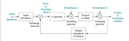
In a closed-loop system there is an *output transducer* or *sensor* which converts the output into the form used by the controller. e.g. Position can be converted to an electrical signal by a potentiometer.
