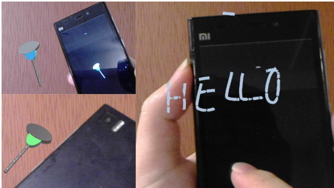
Figure B.1: Virtual Probe controlled by the gyroscope located in the mobile phone. Remote drawing can also be achieved by drawing on the screen of the phone.
